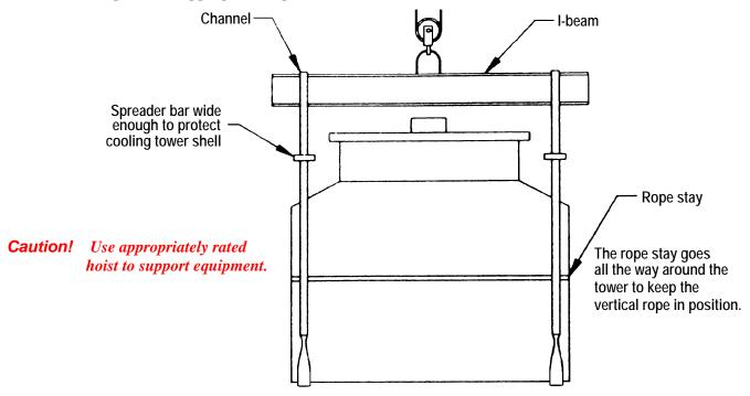
Do not let the rigging transfer any load to the cooling tower shell. Provide support to the bottom of the cooling tower when rigging. Do not rig from the corners of the optional base. Do not rig less than 8 inches from the corners.
